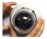
• Snap the dome cover over the camera module.
