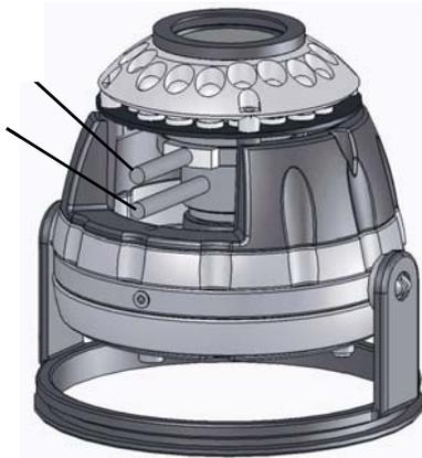
A. Set the zoom lever to the desired position by moving the Zoom lever.
