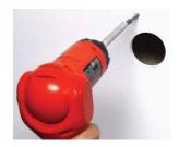
2 Drill holes into the drywall and insert the drywall mounts into the holes
