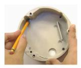
Use the camera's mounting template or your camera to mark the holes as required.
