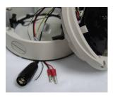
• Pull wires through and make connections.
