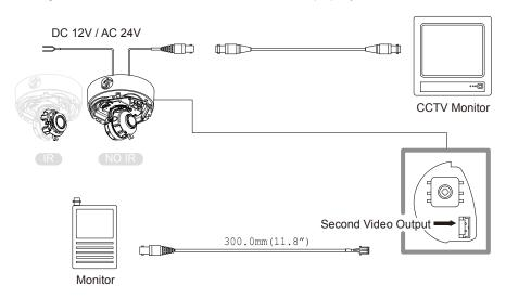
Power Connection: 12VDC & 24VDC Dual Voltage (Auto Polarity Detection and Protection) All cameras are equipped with a second video output for on-site configuration.
