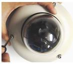
● Tighten the three locking screws in with the L-Wrench to secure the dome cover over the camera
