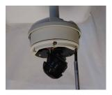
• Attach the camera to the ceiling mount and secure the dome cover properly.
