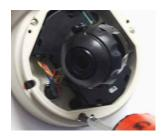
**6** Secure the three (3) assembly screws.
