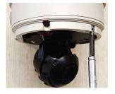
Connect all cables and snap the camera module onto the base
