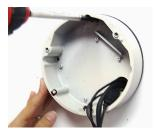
Mount the surface mount base (junction box) to the wall
