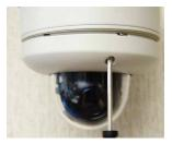
Adjust the camera and secure the dome cover over the camera module
