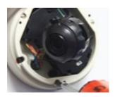
**6** Secure the three (3) assembly screws.
