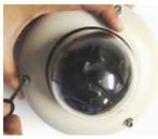
● Tighten the three locking screws in with the L-Wrench to secure the cover dome over the camera
