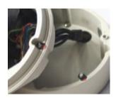
Snap the camera module onto the base by aligning the red and black markings on the base and the camera module.
