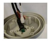
2 Insert the wires from the camera through the wall mount housing.
