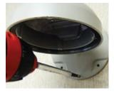
Use the mounting template to make pilot holes. Use the dry wall anchors and woods screws to attach the assembly.
