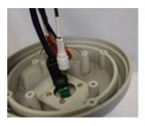
3 Run all necessary cables from the ceiling to the mount.
