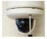
Adjust the camera and secure the dome cover over the camera module.
