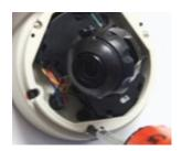
**6** Secure the three (3) assembly screws.
