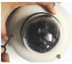
● Tighten the three locking screws in with the L-Wrench to secure the dome cover over the camera
