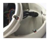
Snap the camera module onto the base by aligning the red and black markings on the base and the camera module.
