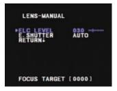
ELC Levels and DC Levels are adjustable. The higher the number, the brighter the image.
