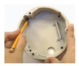
Use the camera's mounting template or your camera to mark the holes as required.
