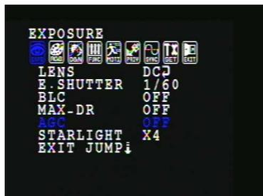
Auto Gain Control automatically adjusts the video gain to enhance picture brightness in low light conditions.
