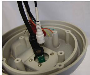
3. Run all necessary cables from the ceiling to the mount.
