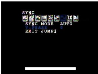
When more than two cameras are installed in a switching system, phase difference in the AC powder line can occur. Therefore, the vertical phase must be adjusted. Select from **0** to **199**.
