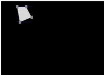
If ON is selected, you can set the area to be masked and the shape and color of the mask. Select SET WINDOW. The masking zone will appear. Press the joystick button to select or deselect the gray squares on the corner(s), then move the joystick left, right, up, or down to adjust the shape of the masking zone. Continue pressing the joystick button to return to the OSD menu. To change the color of the box, select COLOR SET.
