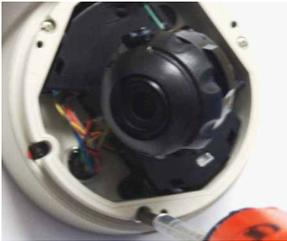
6. Secure the three (3) assembly screws.
