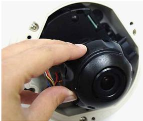
7. Adjust the camera's position by using the 3-Axis Gimbal.
