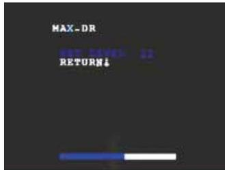
When ON selected, the Max-DR level can be adjusted from 0 to 20.
