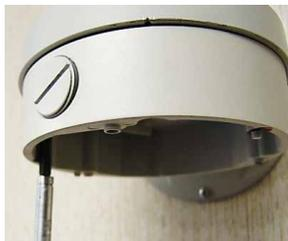
4. Attach the camera's surface mount base (junction box) to the wall mount.
