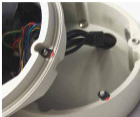
5. Snap the camera module onto the base by aligning the red and black markings on the base and the camera module.
