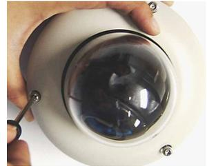
8. Tighten the three locking screws with the L-Wrench to secure the cover dome over the camera.
