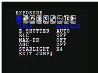
**MANUAL** MANUAL mode supports a Fixed Board lens or a Manual Iris lens.
