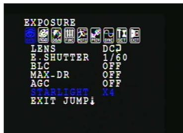
Starlight automatically activates the slow shutter function when a scene is too dark. Adjust the frame integration level from **X2 to X256**.
