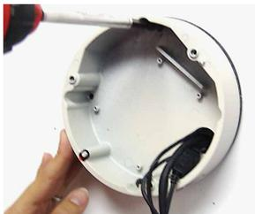
4. Mount the surface mount base (junction box) to the wall.
