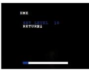
If ON is selected, the HME level can be adjusted from 0 to 60.
