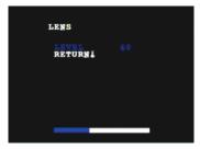
Select DC and control Joystick to adjust the brightness level from 0~99.
