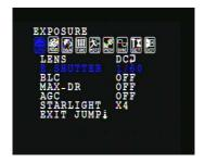
1/60 is the default shutter speed. Select a shutter speed from X256 to 1/100000.
