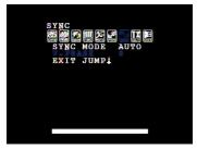
When more than two cameras are installed in a switching system, phase difference in the AC powder line can occur. Therefore, the vertical phase must be adjusted. Select from 0 to 199. Note: This feature is available only when the camera's Sync Mode is set to AUTO.
