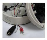
3. Pull wires through and make connections.
