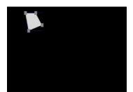
If ON is selected, you can set the area to be masked and the shape and color of the mask. Select SET WINDOW. The masking zone will appear. Press the joystick button to select or deselect the gray squares on the corner(s), then move the joystick left, right, up, or down to adjust the shape of the masking zone. Continue pressing the joystick button to return to the OSD menu. To change the color of the box, select COLOR SET.
