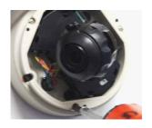
6. Secure the three (3) assembly screws.
