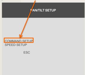
**COMMAND SETUP** 01 CHANNEL PELCO-D MODEL 000 PTZ ID **BAUDRATE** 002400 BPS 1 MSEC CMD DELAY COMMAND PAN/TILT STOP LENGTH 16 CODE 00 00 00 00 00 00 00 00 00 00 00 00 00 00 00 00 **DEFAULT ALL-DEFAULT ESC**
