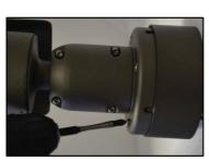
Secure the junction box to a wall or ceiling. Align the camera with the junction box. Secure the camera to the junction box with the included screws.
