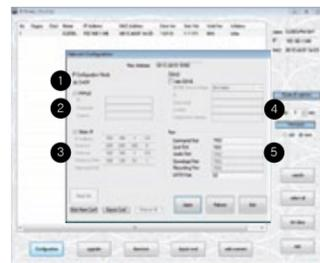
1. DHCP: If DHCP is selected, an IP address will automatically be assigned to the camera. If your network does not support DHCP, a default IP address and subnet mask will automatically be assigned.
