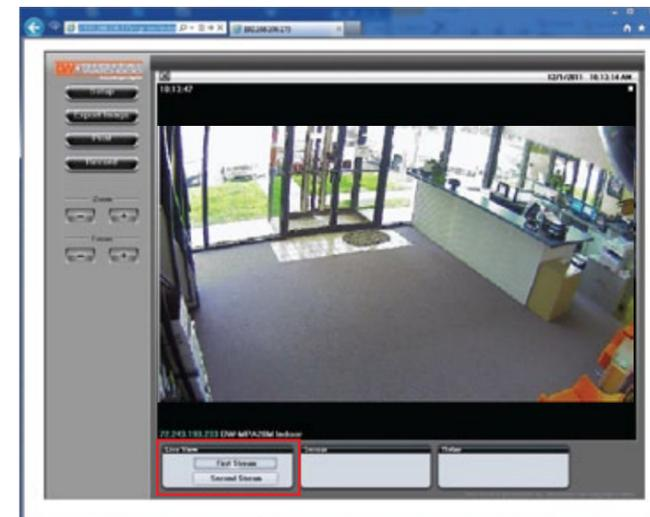
Configure two different stream settings (First Stream and Second Stream) for monitoring and recording. Second Stream is used to record on Motion Detection and the SD card local backup.
