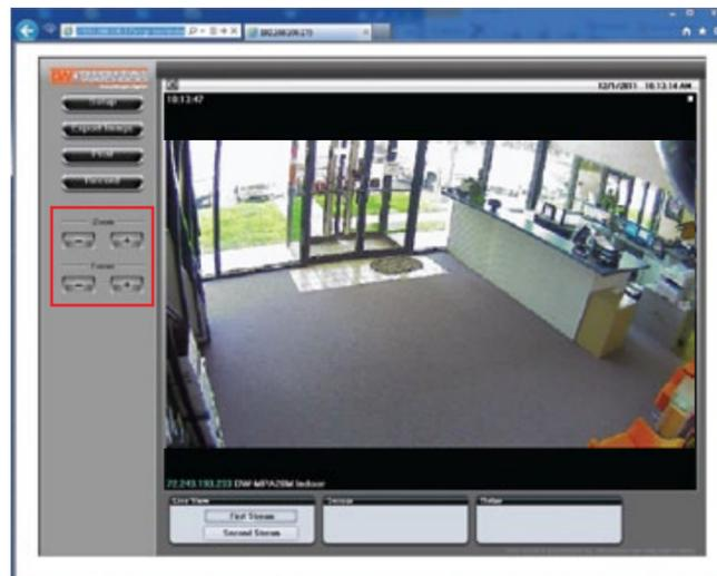
Use the Snapit MEGAPIX camera's remote web viewer to adjust the camera's zoom and focus automatically. Once the configuration is complete, the camera will automatically adjust its focus, zoom, light exposure and lens to match your settings.
