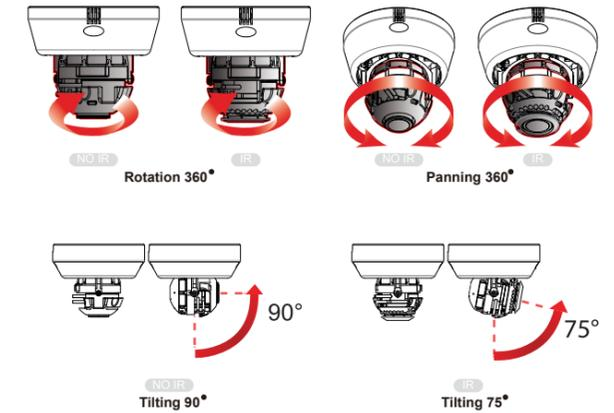
Over-rotating the lens will damage the camera lens module
