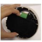
2 While squeezing the plastic dome, hold the camera module and gently remove it from the bubble dome
