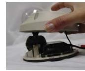
Using the supplied T10-M3x15.0 Allen Key, loosen the four security screws. Carefully remove the dome cover.
