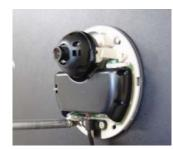
6 Mount the camera to the wall or ceiling using the screws provided with the camera.
