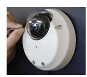
8 Tighten the four locking screws.
