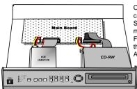
Connect main board and HDD using IDE HDD cable and power cable included in the package. If you install a unit of HDD, jumper Setting of HDD must be on (DS) Master, as specified by HDD manufacturer.
