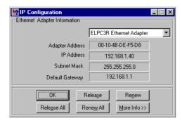
Now, hit the "Release" button and then hit "Renew". If all goes well, you'll get new information, and it is for your DVMR unit. Write down this information on separate paper and input IP Address, Subnet Mask, and Default Gateway into your DVMR to which you want to access via IP network.
