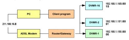
IP forwarding is what we have to set in web site of Router or Gateway to connect external Port to internal IP assigned by Router or Gateway.
