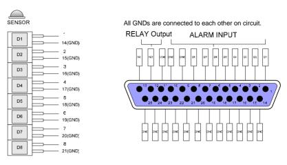
Relay output is output in case there is an alarm input, and is connected to external device using COM-NO (Normal Open) or COM-NC (Normal Close) contact.
