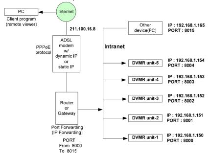
Port forwarding: Port forwarding is called differently by each of router manufacturers, like IP forwarding, IP bounding, port forwarding, port bounding or port routing. Our users can set port forwarding stated in installation manual of router or gateway without big trouble, and complete IP network to which user can connect many of our DVMRs, that are 1 ch DVMR, 4 ch DVMR, 8 ch DVMR and 16 ch DVMR, to access to those units via Internet line far apart from those units.
