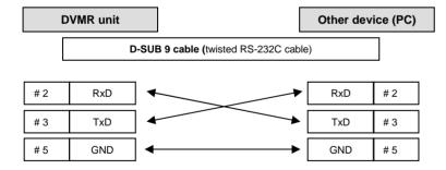
Connection to PC using RS-232C cable
