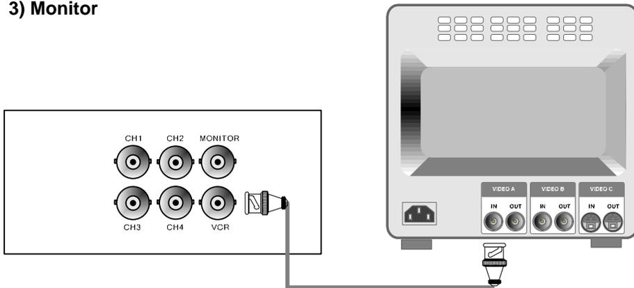
Connect the video output marked MONITOR to Video-In of Main monitor.
