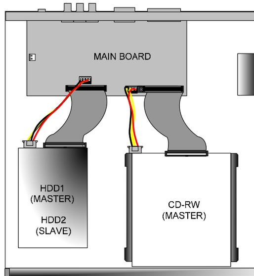
1. Connect Main Board and HDD1 using IDE cable and HDD power cable.
