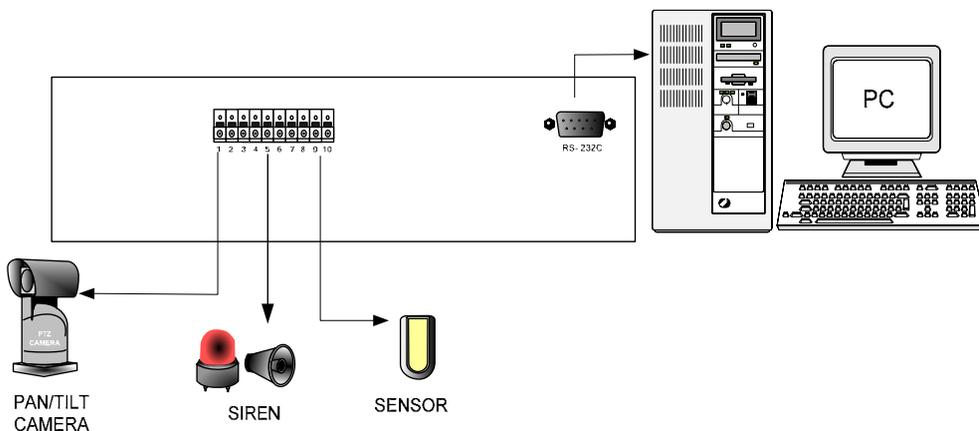
**RS-232C** : Control DVR through RS-232C port by using PC.
