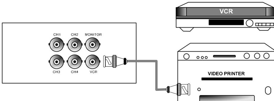
Connect VCR or VIDEO Printer to VCR out on the rear panel of DVR.
