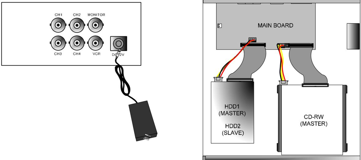
Connect DC 12V 5.83A Adaptor to the back side of Power Jack.
