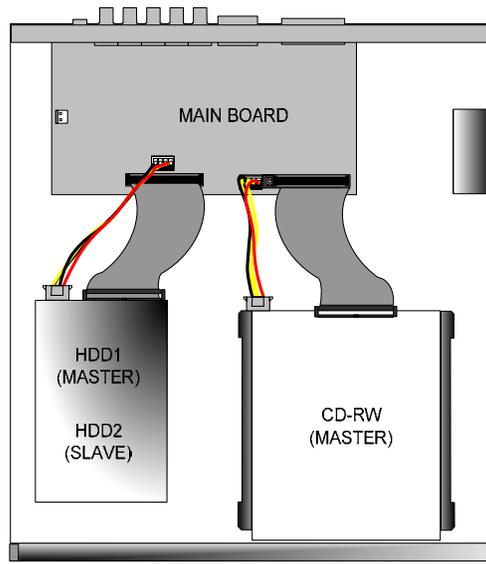
1. Connect Main Board and HDD1 using IDE cable and HDD power cable.
