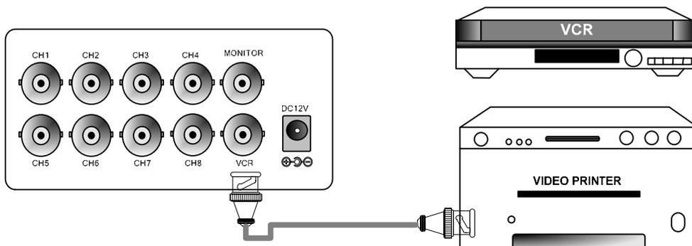
Connect VCR or VIDEO Printer to VCR out on the rear panel of DVR.
