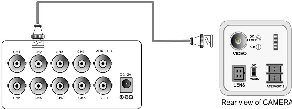
Connect cameras to the camera input on rear panel of DVR marked CAMERA IN.
