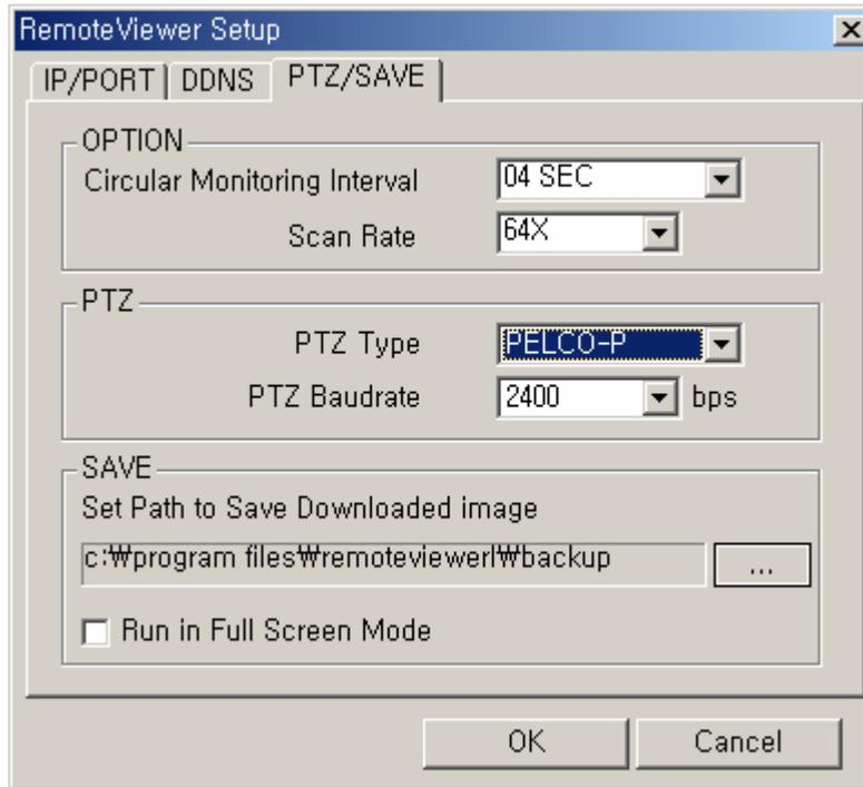
**Circular Monitoring Interval** : This indicates the speed of the channels sequence when the SEQUENCE button is used from the main interface.
