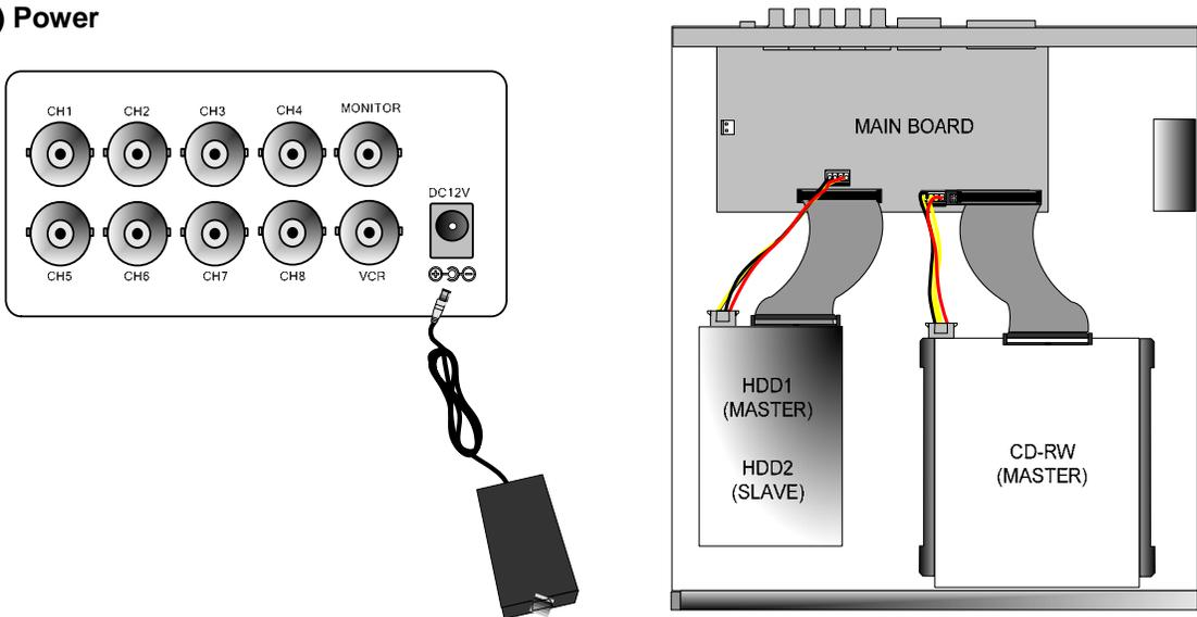
Connect DC 12V 5.83A Adaptor to the back side of Power Jack.
