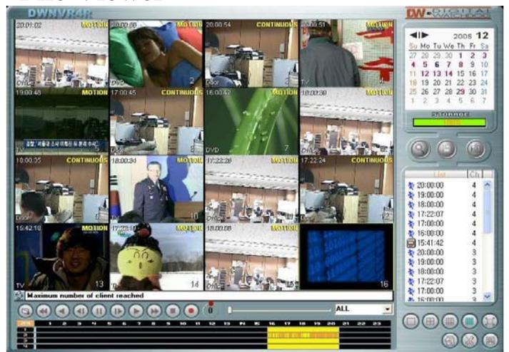
The file viewer mainly consists of image display panel, playback control panel, intelligent time-map panel, calendar, file list panel and display mode panel, etc.
