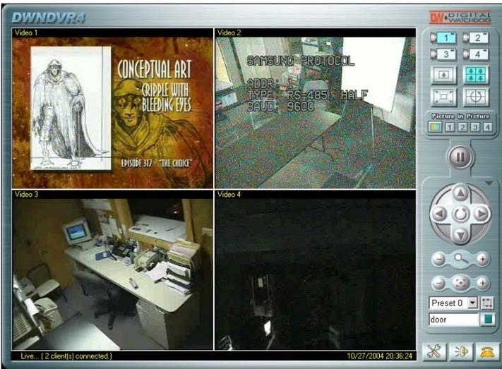
Run Internet Explorer 4.0 or higher on the user's PC, enter DWHVT IP address you want to connect to and press the ENTER key. The first time you access DWHVT home page, the client viewer software is automatically downloaded and installed to allow you to view the MPEG4 video images. You must have the Active-X Control plug-in installed in your browser. If it is not already installed, you will be prompted to do so at this time.
