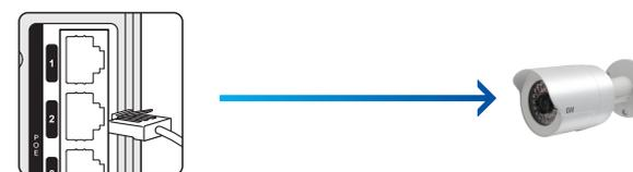
1. Connect the network camera directly to the PoE port of the NVR.
