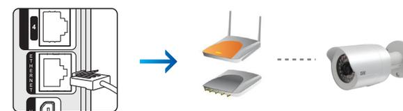
1. Connect the network camera to the NVR, using a hub, a router or switch.
