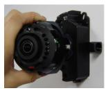
Adjust the camera lens position by using the 3-Axis Gimbal
