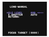
ELC Levels and DC Levels are adjustable. The higher the number, the brighter the image.
