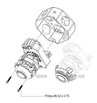
**NOTE**: Screws required for electrical junction boxes are not supplied. These screws are readily available at well-stocked electrical supply store.
