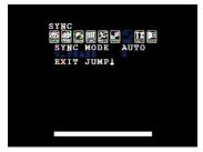
When more than two cameras are installed in a switching system, phase difference in the AC power line can occur. Therefore, the vertical phase must be adjusted.
