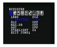
1/60 is the default shutter speed. Select a shutter speed from X256 to 1/100000.
