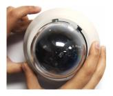
Snap the dome cover over the camera module.
