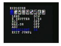
Starlight automatically activates the slow shutter function when a scene is too dark. You can adjust the frame integration level from **X2** to **X256**, or select **OFF**.
