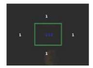
When BLC is enabled, adjust the BLC Level in five areas in the screen. Each can be adjusted from 0 to 255. Move the joystick controller LEFT and RIGHT to adjust the values in each area. Move the joystick controller UP and DOWN to switch between areas. When all adjustments have been made press the joystick controller to return to the main menu.
