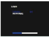
Select DC and control Joystick to adjust the brightness level from 0~99.
