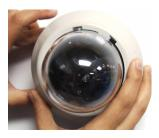
Adjust the camera lens, and snap the dome cover over the camera module.
