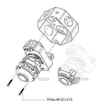
**NOTE**: Screws required for electrical junction boxes are not supplied. These screws are readily available at an electrical supply store.
