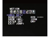
The camera can detect the movement and display an alarm on the screen when movement is detected.
