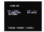
ELC levels and DC levels are adjustable. The higher number, the brighter the image.
