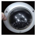
Secure the dome cover to the camera base by using the assembly screws. Make sure the camera is tightly secured to avoid damage to the camera module.
