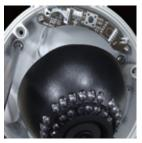
Pull wires through and make connections. Refer to page 9. Use mounting template to mount camera with dry wall mounts and wood screws.
