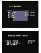
If MANUAL is selected, you can adjust the BLC levels in four areas of the scene (Top, Bottom, Left, Right). Increase the BLC levels to make the image brighter.
