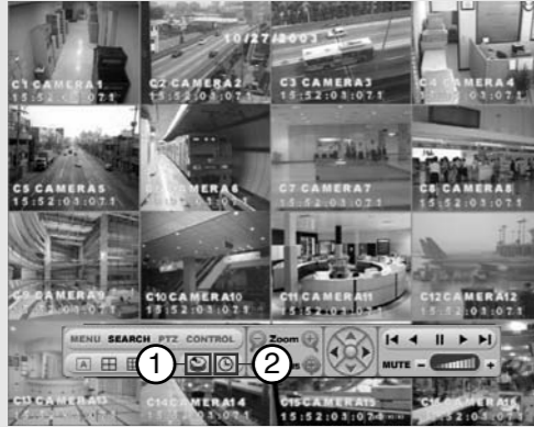
[Figure 3-3. Mouse pop-up menu on multiple channel playback screen]
