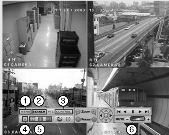
[Figure 3-1. Pop-up menu operated by mouse on surveillance mode]
