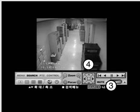
[Figure 3-4. Mouse pop-up menu on single channel playback screen]
