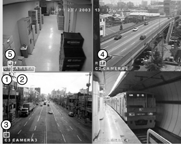
[Figure 2-1. Main Surveillance Mode by 4 split screen]
