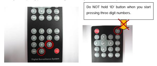
3) When you hear the beep sound when pressing the last third digit number, the REMOTE ID setup is completely done.
