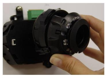
3. Adjust the camera's position using the 3-Axis Gimbal.
