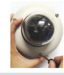
Tighten the four locking screws in with the L-wrench to secure the cover dome over the camera.
