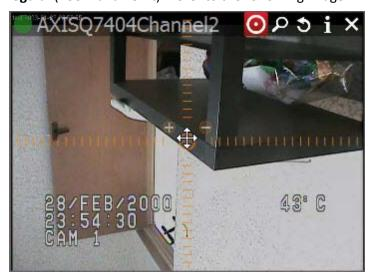
Use + and - buttons to zoom in/out. **Left-Click** on the center circle, **Hold Left Mouse Button** and **move the cursor** to move **Camera** to the desired position.
