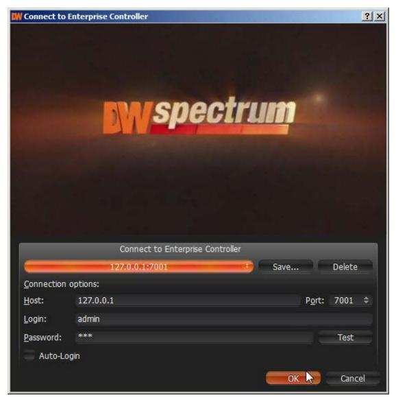
DW Spectrum provides a powerful mechanism that can auto-discover **Enterprise Controllers** in **local network**. The easiest way to connect to EC is to use one of the auto-discovered EC.
